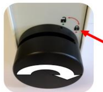
Closed and locked protecting casing (seals)
